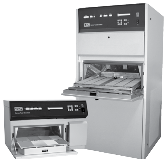
Q-SUN Xenon Test Chambers reproduce the full spectrum of sunlight, including ultraviolet, visible light and infrared.
