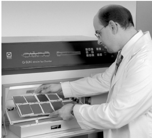
The Q-SUN Xe-1 allows for versatile specimen mounting, including 3-D parts and flat panels.
