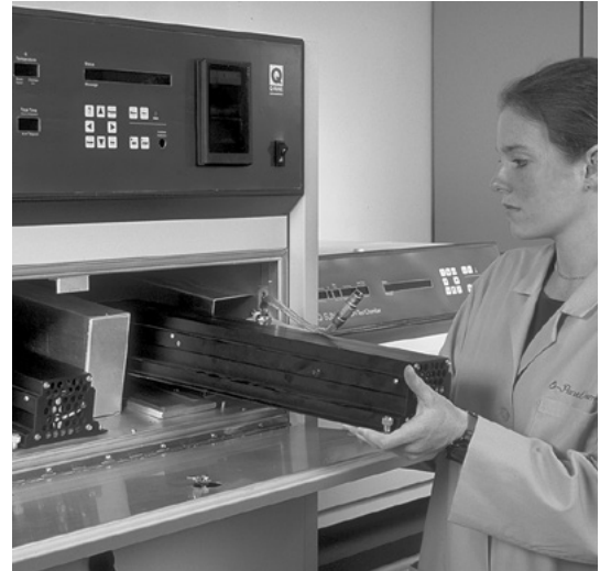
Q-SUN chamber lamp replacement is almost effortless: just open the hinged door, disconnect and slide out the lamp.
