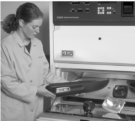
The Q-SUN Xe-3 accommodates 3-D parts, test tubes and petri dishes in addition to flat panels.
