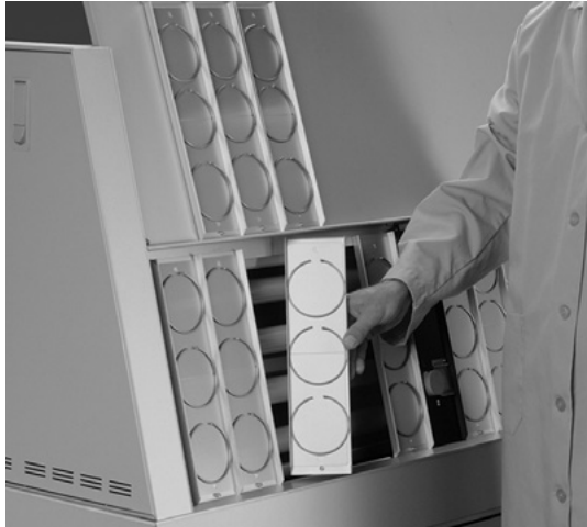
A QUV tester has five times the capacity of the Q-SUN Xe-1 and 1.5 times the capacity of the Xe-3.
