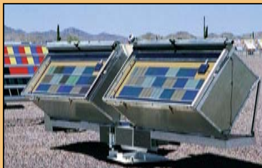
These AIM Boxes in Arizona are used to test materials for automotive interiors. They can hold large, 3-D parts like instrument panels.
