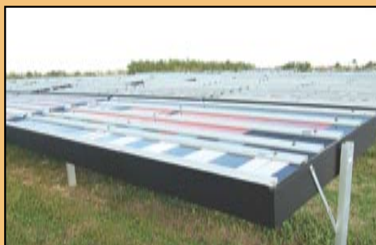
High temperatures are a major factor in Florida exposure tests. Using a black box increases the temperature of the specimens even more.
