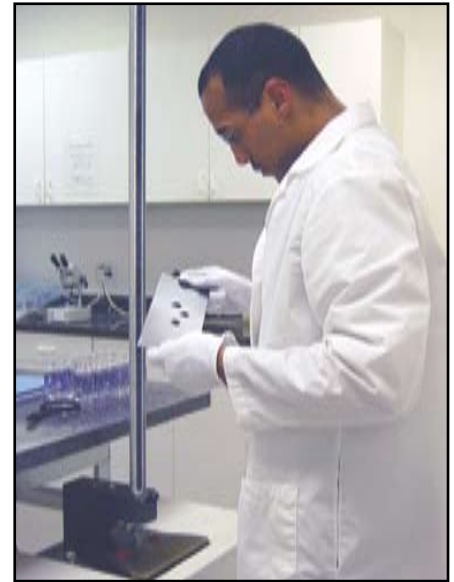
Impact testing at Q-Lab Florida.
