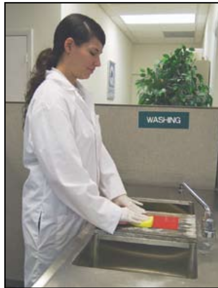
Washing specimens ensures that surface contaminants will not affect test results.
