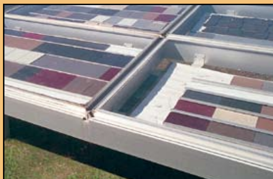
Sub-frames with window glass protect interior materials tested in “under glass” exposures at Q-Lab Arizona.
