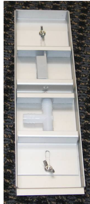
3.25 inch wide x 0.7 inch deep specimen holder with adjustable mounting clamps V-4019-X
