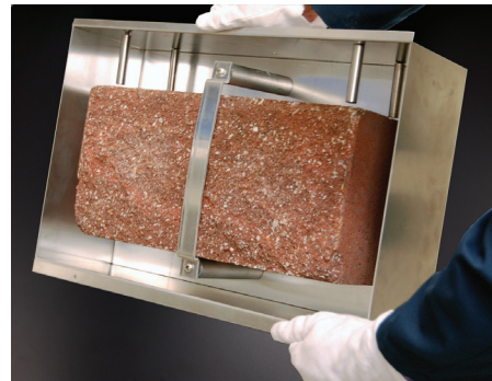
Adding brackets and other modifications allow further versatility to hold even very heavy samples, such as concrete blocks.
