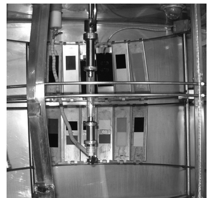
Rotating-drum specimen holders accommodate flat specimens.
