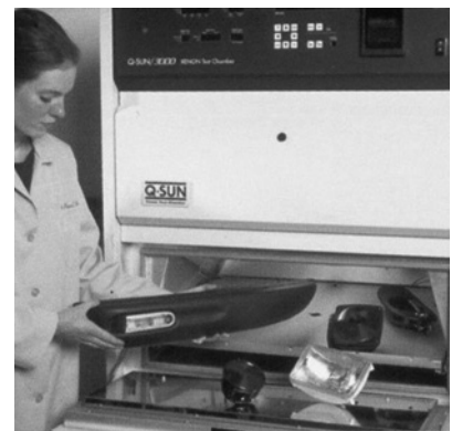
The Q-SUN accommodates flat and 3-dimensional parts.
