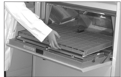
The Q-SUN's slide-out specimen tray makes specimen mounting fast and easy
