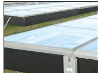
Under glass black box exposure systems, used for automotive interior materials.
