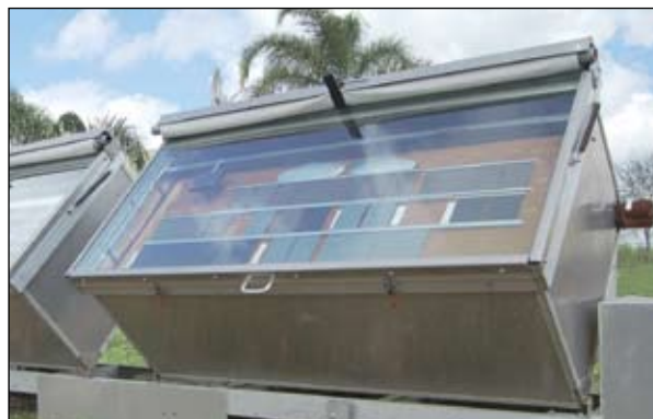
Q-Lab Weathering Research Service offers both typical direct exposure testing and special services. Shown above are AIM (automotive interior materials) boxes, designed to simulate the environment inside an automobile.
