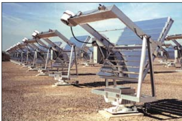
Q-Trac Natural Sunlight Concentrators at Q-Lab Arizona provide accelerated natural weathering results.
